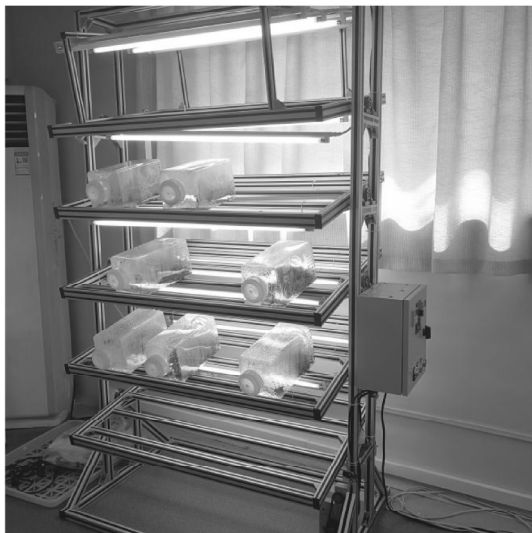
图1 摇摆式间歇浸没生物反应器 Fig.1 Swinging type temporary immersion bioreactors system
